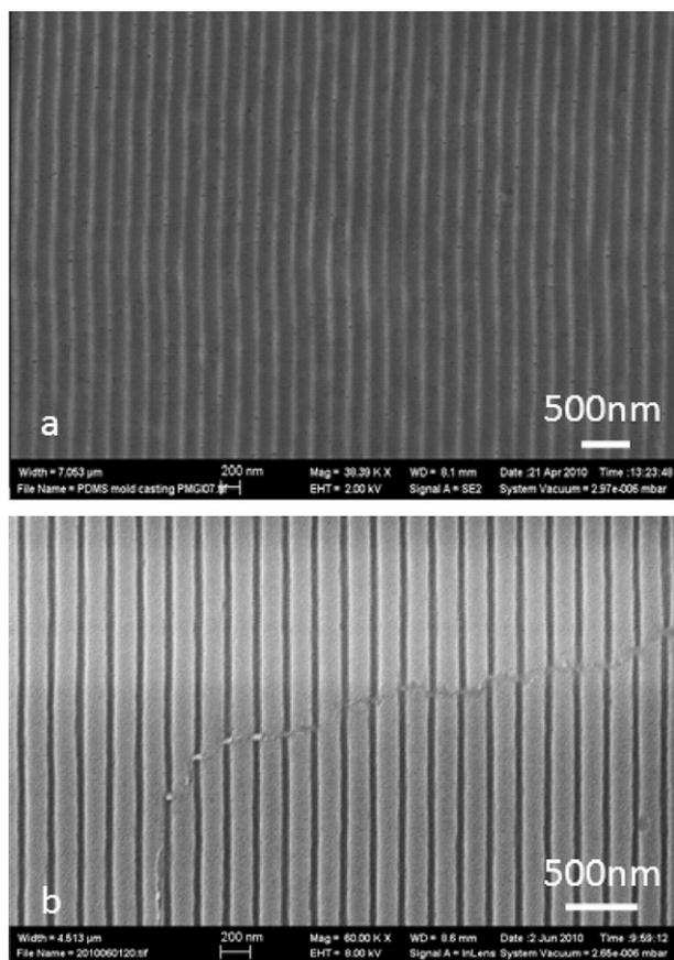
**Fig. 2.** (a) SEM image of a mold in UV-cured resist on PDMS duplicated from a PMGI sacrificial mold that was patterned using the method as shown in Fig. 1a; (b) SEM image of a grating imprinted into UV-curable resist using this mold.
