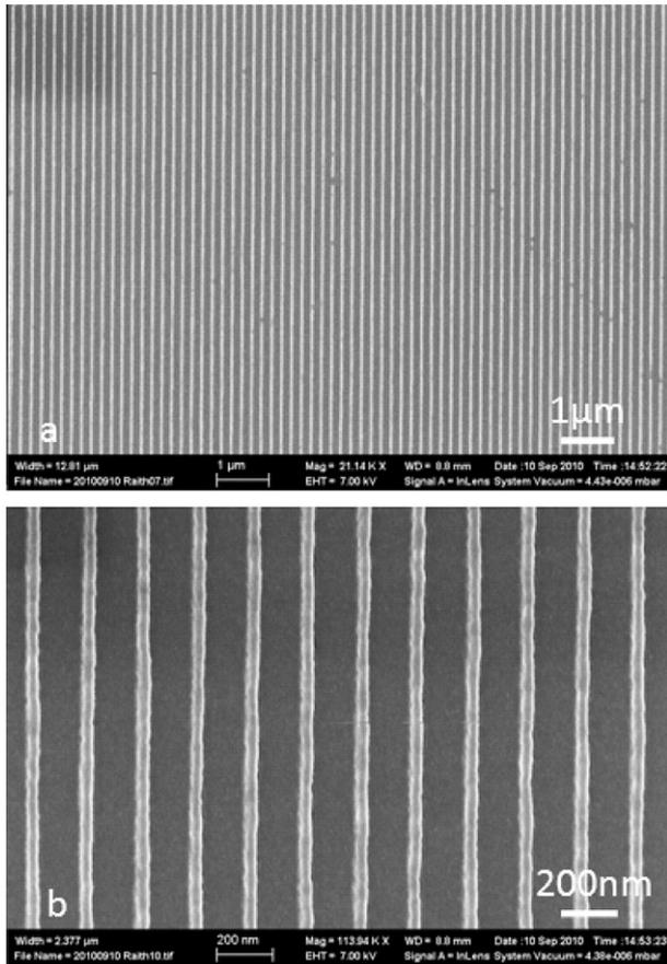
**Fig. 3.** SEM image of a grating imprinted into UV-curable resist using a mold in UV-cured resist on PDMS, which was duplicated from a PMGI sacrificial mold that was patterned using the method as shown in Fig. 1b. (a) Overview; (b) zoom-in image.
