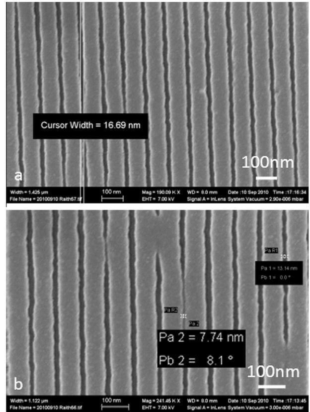
**Fig. 4.** SEM image of a grating imprinted into UV-curable resist using a mold duplicated from a PMGI sacrificial mold that was patterned using the method as shown in Fig. 1c. (a) Grating of 100 nm period with a trench-width ~17 nm; (b) a collapsed grating shows features down to 8 nm.
