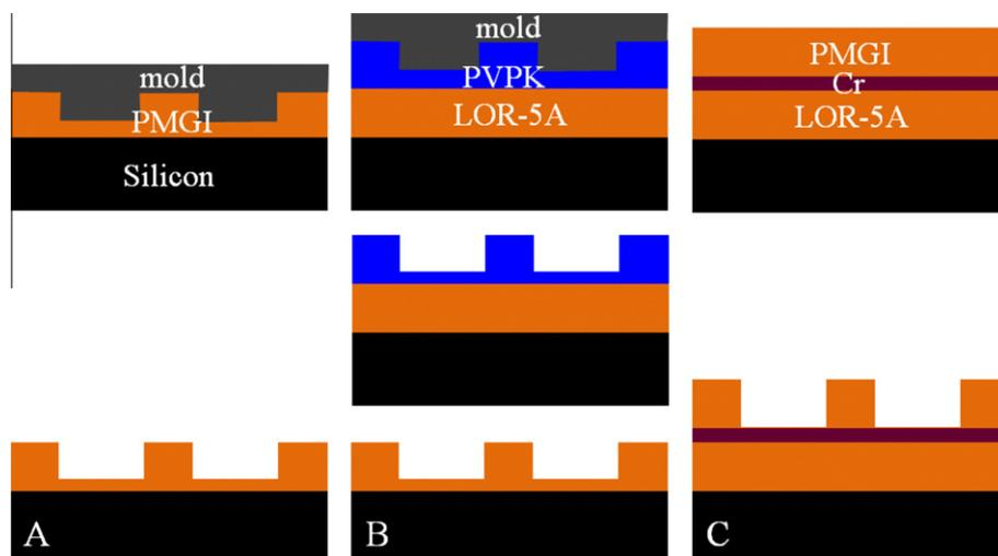
**Fig. 1.** Three methods for the fabrication of sacrificial mold in PMGI (or LOR-5A that is based on PMGI). (A) Direct imprint into PMGI at high temperature; (B) imprint into PVPK at reduced temperature, then RIE transfer the pattern into LOR-5A; (C) electron beam lithography using PMGI as positive resist.
